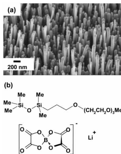
Figure 1. Structures of nanofibers and electrolyte components. (a) Scanning electron microscope (SEM) image of vertically aligned carbon nanofiber electrode. (b) Structures of organosilicon electrolyte and of the lithium salt. Upper panel: 1-(3-{2-[2-(2-Methoxy-ethoxy)-ethoxy]-ethoxy}-propyl)-1,1,3,3,3-pentamethyl-disiloxane (2SM3). Lower panel: Lithium bis-oxalato-borate (LiBOB).
